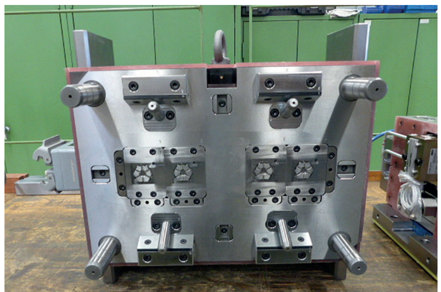
Fig. 5. 4-cavity mold (moving half) for a stator, which runs on a round-table machine.
